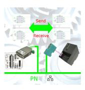
Coupling S7-controller with MPI/Profibus at S5-control with PD-port via network
