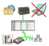
S5-PLC triggered DB-backup/-restore without additional PC via PG-socket and Ethernet on FTP-server
