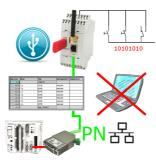
Via digital input triggered DB-backup/-restore without additional PC via PG-socket and Ethernet to USB-stick
