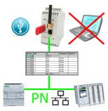
S7-PLC triggered DB-backup/-restore without additional PC via PN-port to USB-stick
