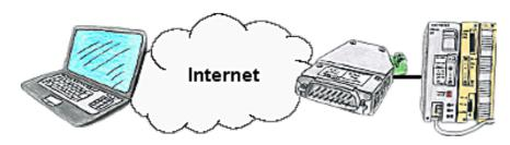
You have access to a on-site network and your PLC has no LAN-connection? No problem, plug the S5-LAN on the PLC and you will have immediate access to the PLC from afar.
