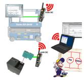
Use the latest S7-TCP-IP panels for your MPI / Profibus. Thanks to WLAN also usable for mobile platforms or cranes. Connect several nodes at the same time via a network module. Simultaneous access from different systems possible.
