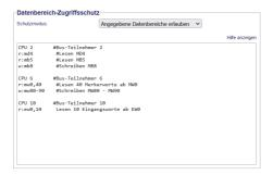
With the management of the data-areas it is determined whether the entered data-areas can be read/written via the module with the connected controllers. A central button for the function determines whether the specified inputs are "allowed" or "not allowed" are.
