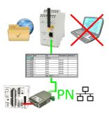
S5-PLC triggered DB-backup/-restore without additional PC via PG-socket and Ethernet on FTP-server
