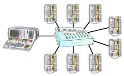
You have many PLC and you want to programm them central on one place? No problem, you have to connect them all to the KOR/MUX-Tele-Switch an with the PD-bus-selection of your Step5-software you go ONLINE. Of course the KOR/MUX-Tele-Switch is cascadable, so you can connect up to 30 PLCs to the devices.
