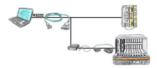
You have a PC with programming software and a 9pin COM-port as interface? No problem, for this purpose the PG-UNI-II-cable is exactly the right product. Connect it to PLC and PC and you're Online. The communication itself is visible by the both included LEDs. Even the 25pin interface of the AS511-card is no problem. You need the NETZ-adapter and also the AG-150-adapter and then this control is programmable, too.
