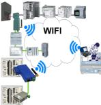
Wired or wireless communication (WIFI) via the same adapter with the respective control Devices from the BRIDGE-family always connect a wired-network with a wireless-network (WIFI) and a specific PLC-interface. This gives you access to the directly connected controller via WIFI (with S7 to the entired bus) as well as to the wired Ethernet. Of course also from wired Ethernet to WIFI and control/bus.
