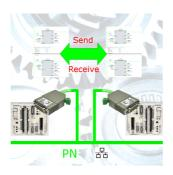
Coupling S5-controller with PD-port at S5-controller with PD-port via network
