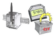
You always need a current time, but do not always have a time-server on site. With the integrated battery-backed RTC you always have the current time in the unit. Even if the power fails, the time in the unit continues to operate, so that when the voltage returns, the time continues to run correctly.
