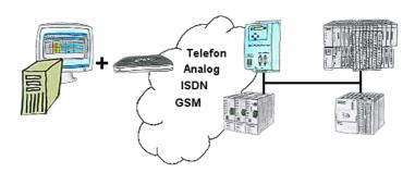
You have to solve a problem in the PLC-program, but the installation is not placed nearby? No problem, start your PG-2000-software with "option teleservice", activate your modem and after selection intra PG-2000-software access to the PLC is possible as if being on-site.
