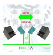
Coupling S7-controller with MPI/Profibus at S7-controller with MPI/Profibus via network
