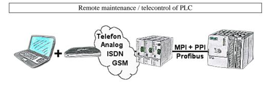
The access to the connected PLC with the Siemens TS-software or PG-2000 including TS-option results of coupling via Analogue-, ISDN- (only with AB-adapter) as well as GSM-line.
