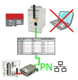
$\ensuremath{\mathsf{S5-PLC}}$  triggered DB-backup/-restore without additional PC via PG-socket and Ethernet on SD-card
