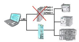
Do you have a PLC without CP343-1 or CP443-1 and a TP-II as remote maintenance device? Then activate the CP-mode of the TP-II and your visualisation goes directly ONLINE via the LAN of the TP-II.
